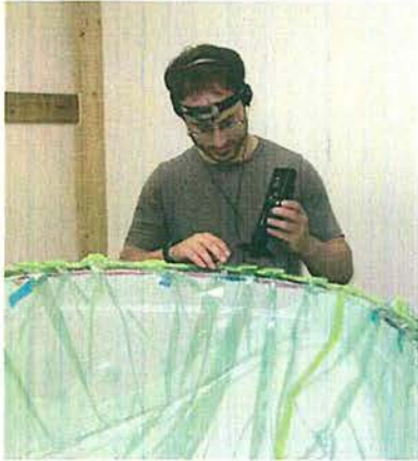
Ultrasonic Leak Checks
